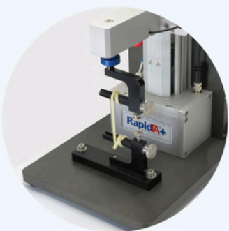
Noodle stretching rig
